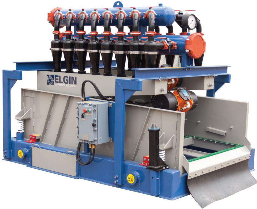
With the combination of a desander and desilter mounted over a powerful multi-functional Hyper-G™ shaker, Elgin’s line of mud cleaners offer both high performance and versatility for the operator. This integration of advanced equipment puts forth a unit that can handle large volumes of circulating fluids and is able to retain fluid integrity.
